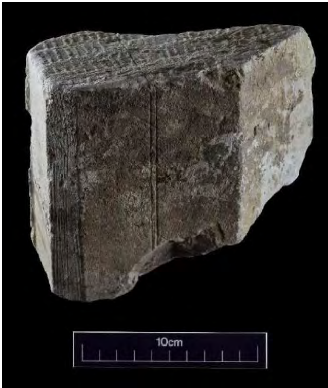
Fig. 5 Voussoir stone showing claw tooling (© Allen Archaeology/The National Trust)
