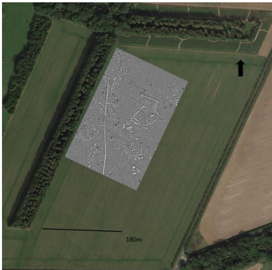
Fig. 4 St Clair's Farm: linear greyscale image of the minimally processed magnetometry data superimposed over Google Earth aerial photograph
