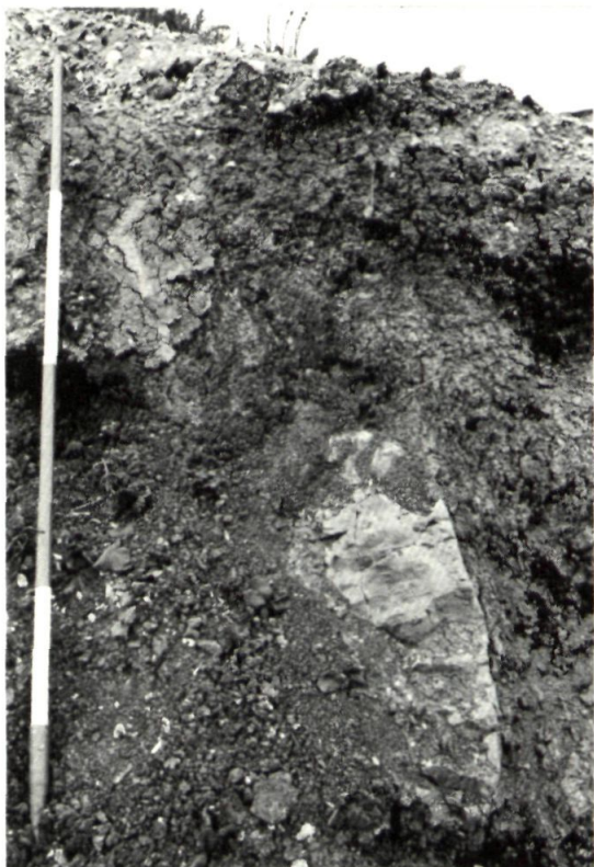
Fig 3. Naish Farm. Photograph of part of the presumed valley bulge structure showing the up-ended nodular concretion. The distorted shelly lens (pale grey) can be seen above and to the left of the nodule (just to the right of the ranging rod). The ranging rod is marked in \frac{1}{2} m divisions. This photograph should be compared with the sketch in Fig 2.
