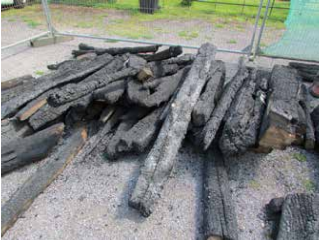
Fig. 2. Timbers from the fire set aside for possible dendrochronology (photo Margaret Bennett).
